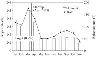
Fig.8 Trainsition rate of out of grade
