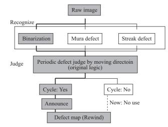
Fig.6 Logic of defect recognition
