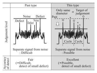
Fig.4 The most suitable condition of judgement level
