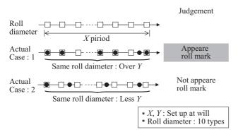
Fig.3 Judgement mechanism of roll mark
