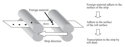
Fig.1 Mechanism of roll mark
