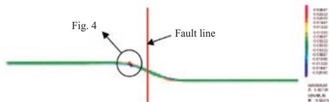
Fig.6 Deformation of a buried pipeline (Fig.2)
