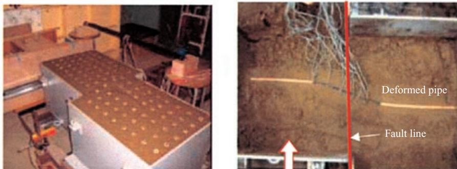
Fig.5 Bending of a buried pipeline due to shear deformation
