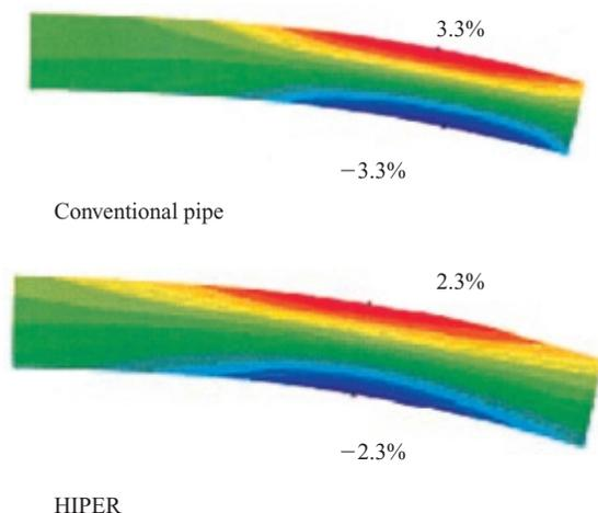
Fig.7 Comparison of strain distribution of buried pipeline
