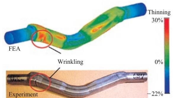
Fig.2 Comparison of results between an FEA and an experiment (Case 1)
