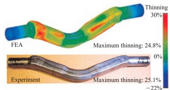
Fig.3 Comparison of results between an FEA and an experiment (Case 2)
