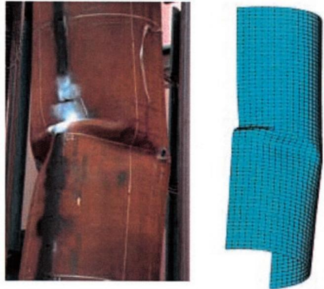
Fig.4 Shell wrinkling due to bending
