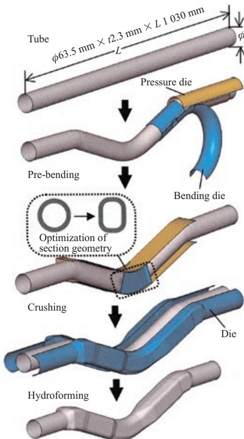
Fig. 1 Process of tube hydroforming
