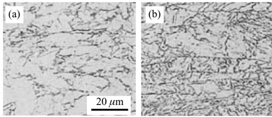
Photo 1 Examples of microstructure of extremely-low carbon bainitic steel (a) YS = 485 MPa (b) YS = 535 MPa
