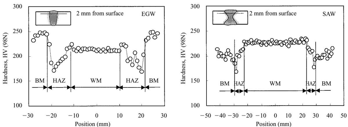
Fig.4 Hardness distribution of the welded joints
