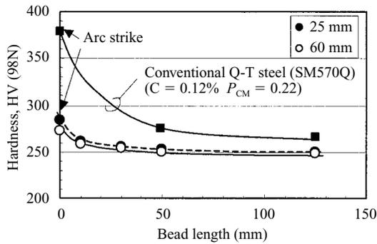
Fig.3 Result of maximum hardness test
