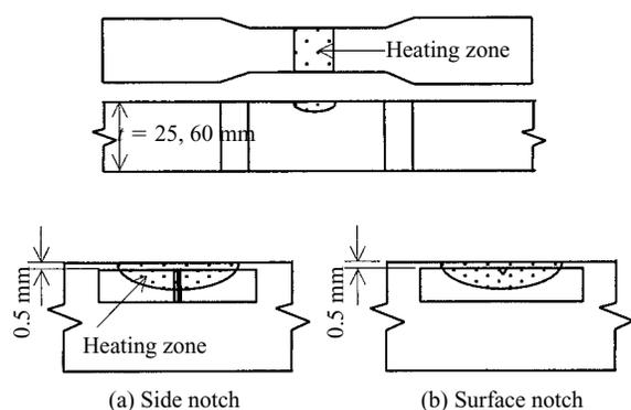
Fig. 2 Preparation of tensile test specimen and location of V-notch Charpy impact specimen
