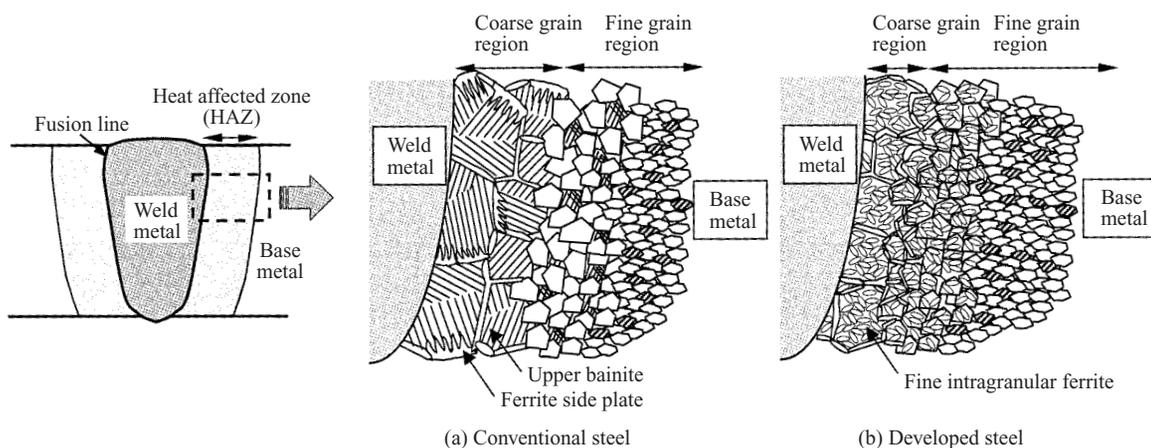
Fig.1 Schematic diagram of high heat input welded joint
