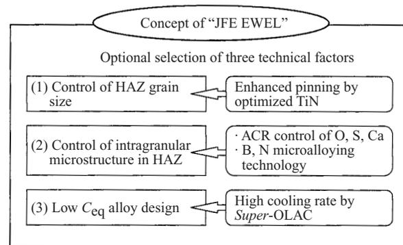
Fig.2 Concept and technical factors of HAZ toughness improvement in “JFE EWEL” for high heat input welding
