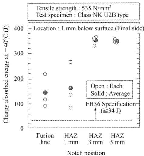
Fig. 6 Mechanical properties of arc welded joint of YS355 N/mm<sup>2</sup> class F grade plate
