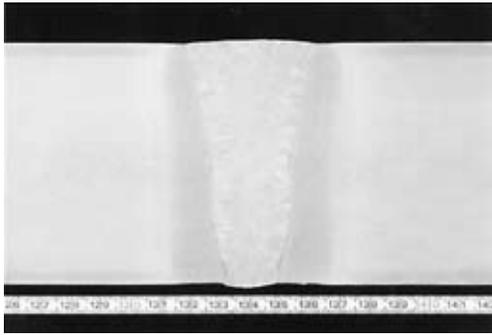
Photo 3 Macrostructure of YS390 N/mm<sup>2</sup> class welded joint (Electro-gas arc welding, heat input = 680 kJ/cm)
