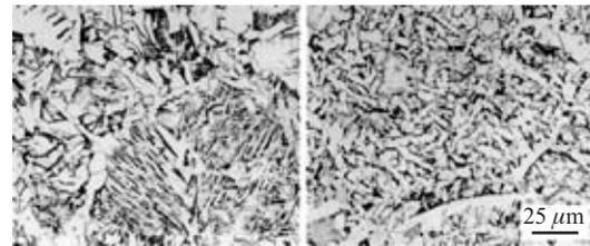
Photo 2 Microstructure of simulated HAZ (Peak temperature: 1 400°C, cooling time from 800°C to 500°C: 390 s)
