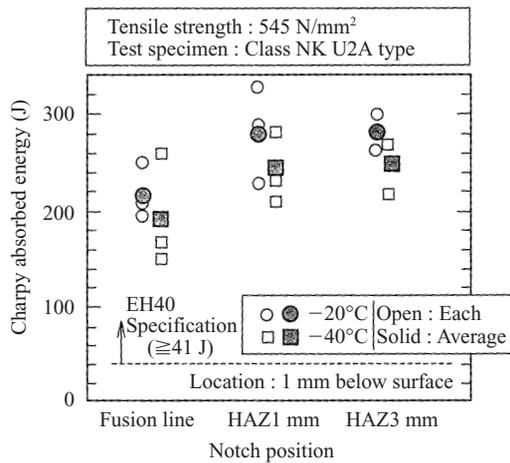
Fig. 5 Mechanical properties of electro-gas arc welded joint of YS390 N/mm<sup>2</sup> class plate
