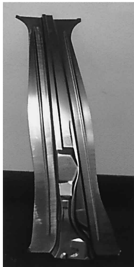
Photo 7 Applied example for center pillar reinforcement of TS980 MPa steel sheet (low YR type)(Formed by the experimental stamping tools in JFE Steel)
