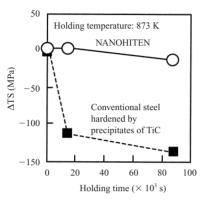
Fig.3 Comparison in thermal stability of strength between NANOHITEN and conventional HSLA steel
