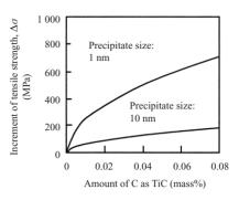
Fig.2 Effects of size and amount of precipitates on the increment of tensile strength
