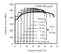
Fig.6 Stress-strain curves for TS 440 MPa grade BHT steel with different amount of prestrain after strain aging
