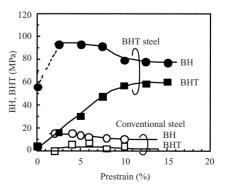
Fig.7 Effect of prestraining on BH and BHT values for BHT steel after strain aging (t = 1.4 mm)
