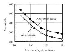
Fig.8 Influence of strain age hardening on fatigue strength for BHT steel
