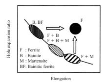
Fig. 1 Effect of microstructure on elongation-hole expansion ratio balance
