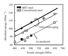
Fig.9 Comparison in absorbed energy under high strain rate tensile testing between BHT steel and conventional steel
