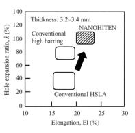
Fig.4 Comparison of El-λ balance in 780 MPa grade hot-rolled steels
