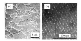
Photo 1 Microstructure(a) and precipitates(b) of NANO-HITEN
