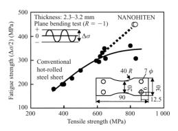
Fig.5 Comparison of fatigue strength between NANO-HITEN and conventional HSLA steel
