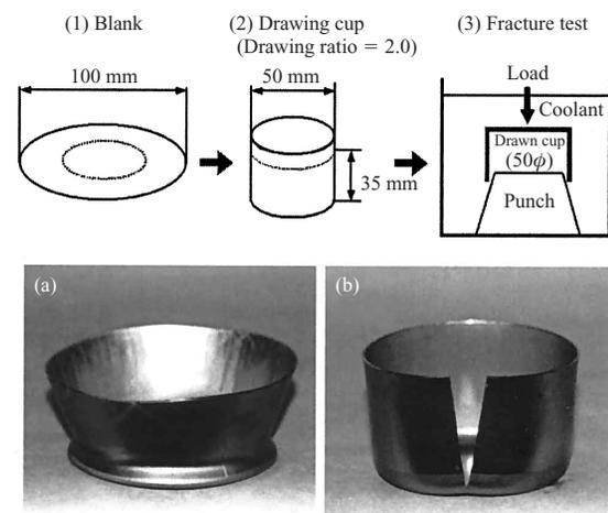
Photo 5 Schematic diagram of evaluation method of the transition temperature for secondary-work-embrittlement; (a) Non-brittle fracture, (b) Brittle fracture
