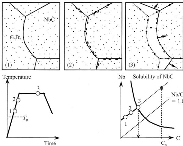
Fig. 6 Schematic illustration exhibiting the hypothesis on the mechanism of PFZ formation in steel B
