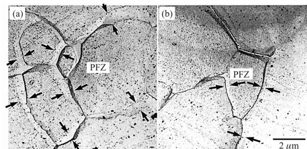
Photo 4 TEM replica micrographs of annealed specimens with the heating rates of (a)  $2^{\circ}\text{C/s}$  and (b)  $15^{\circ}\text{C/s}$
