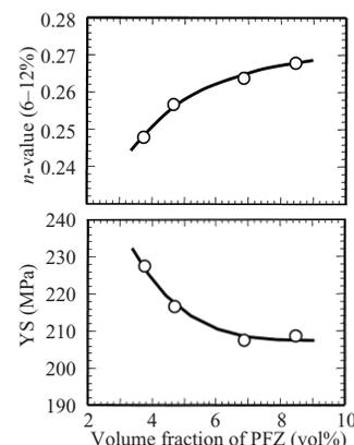
Fig. 8 Effect of volume fraction of PFZ on mechanical properties of annealed specimen
