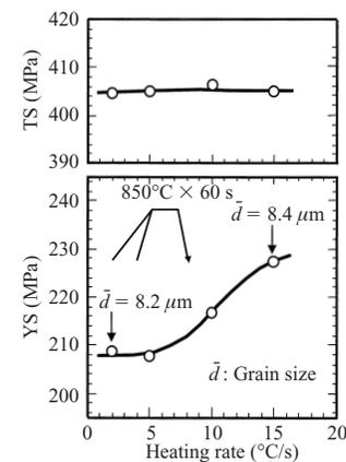
Fig. 7 Effect of heating rate on mechanical properties of the steel annealed at  $850^{\circ}\text{C}$  for 60s
