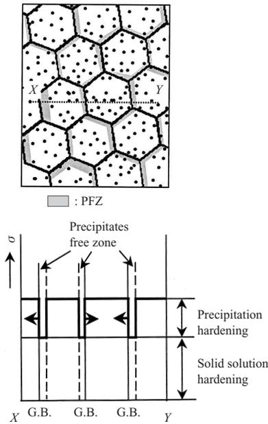
Fig. 5 Schematic illustration showing the hypothesis on the mechanism for lower yielding in steel B strengthened by the solid-solution elements and fine Nb precipitates with PFZ
