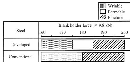
Fig. 10 Press-formability for a front fender model of the developed 440 MPa galvannealed steel sheet and the conventional galvannealed IF-HSS
