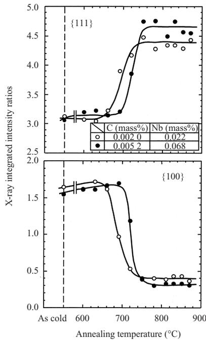
Fig.3 Change in normalized X-ray integrated intensity ratio with annealing temperature for steels A and B
