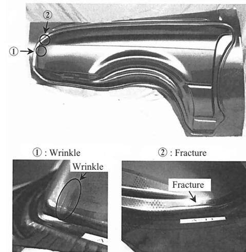
Photo 6 Front fender model for evaluating press-formability
