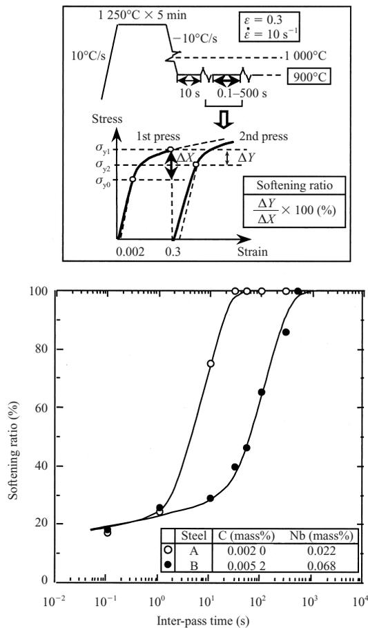
Fig. 1 Change in softening ratio with inter-pass time during hot compression at 900°C for steels A and B
