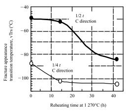
Fig.7 Influence of reheating time at forging on vTrs
