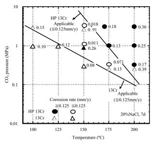
Fig. 16 CO<sub>2</sub> corrosion map for 13Cr and HP13Cr
