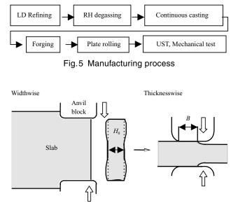
Fig.6 Schematic diagram of CC slab forging
