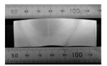
Photo 2 ERW weld seam of 1.000" thick pipe (Nital etched)
