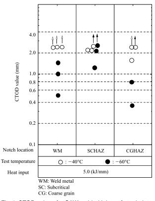
Fig.4 CTOD values for SAW welded joints of steel plate developed
