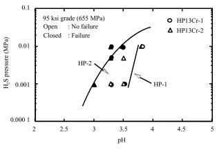
Fig. 17 SSC test result for HP13Cr pipe
