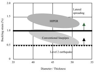
Fig.9 Critical buckling strain of HIPER
