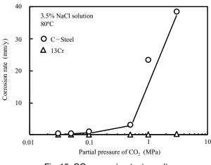
Fig. 15 CO<sub>2</sub> corrosion test result
