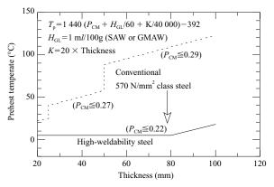
Fig.2 Example of the decrease in required pre-heat temperature for low  $P_{\rm CM}$  HSLA steel plates<sup>2)</sup>
