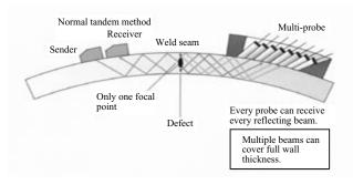
Fig. 13 Schematic image of JFE Steel's new multi-probe system compared with normal tandem method
