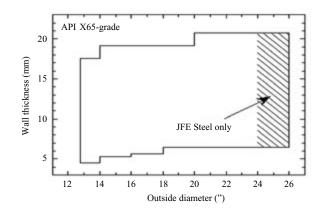
Fig.11 Available manufacturing size range of X65-grade ERW linepipe of JFE Steel at 26" ERW mill
