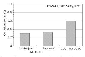
Fig.18 CO<sub>2</sub> corrosion test results of KL-12CR welded joint
