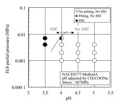
Fig. 19 SSC test results of KL-HP12CR welded joint
