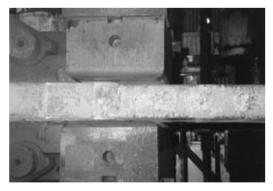
Photo 1 Forging reduction in thickness of CC slab
