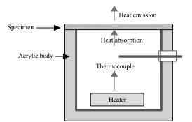
Fig.2 Radiation performance tester
