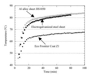
Fig.1 Temperature increase inside a radiation tester
