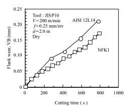
Fig.14 Comparison of flank wear between NFK1 and AISI 12L14
