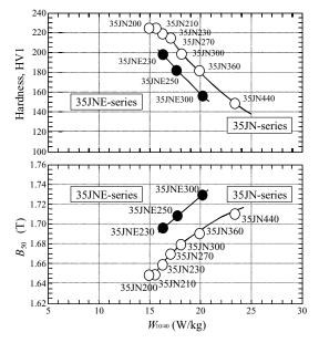
Fig.7 Magnetic and mechanical properties of JNE and JN series
