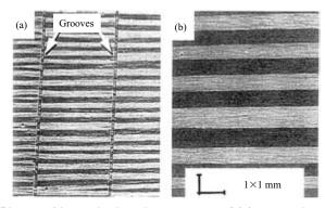
Photo 4 Magnetic domain structures of (a) grooved and (b) plain materials observed by type-II Lorentz SEM method
