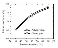
Fig.9 Effect of core assembly method on efficiency of model motor using 50JN700\*B as core material
