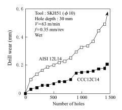
Fig. 15 Comparison of drill machinability between CCC12C14 and 12L14
