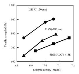
Fig.16 Relations between sintered density and tensile strength of sintered compacts made of KIP 21SX and SIGMALOY 415S
