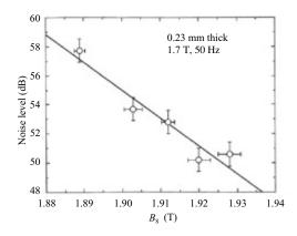
Fig.4 Relation between noise level of step-lap model transformer core and *B*<sub>8</sub> value of core material
