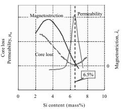
Fig.19 Variation of magnetic characteristic by Si content of Fe-Si alloy
