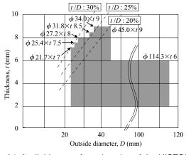
Fig.24 Available manufacturing size of the HISTORY steel tube
