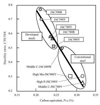
Fig.5 Relationship between ductility ratio, CTS/TSS and carbon equivalent,  $P_{\rm CM}$  at welding current of 7.5 kA
