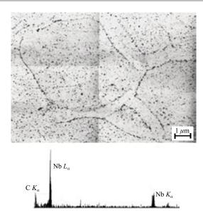
Photo 2 TEM image with replica and EDS spectra of precipitates observed in SFG-Hiten
