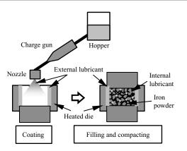
Fig.29 Schematic diagram of warm compaction method with die wall lubrication
