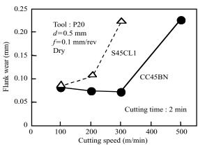
Fig.28 Comparison of flank wear
