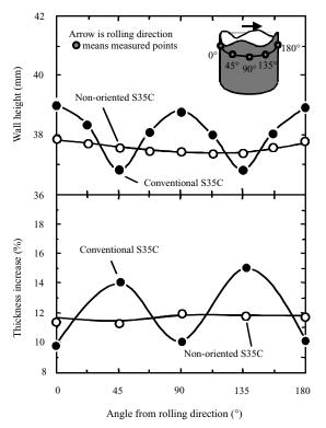
Fig.7 Change in wall height and wall thickness after cup cylinder deep drawing
