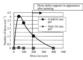
Fig.9 Number of dross on galvanized steel sheet
