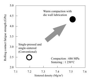
Fig.30 Relation between sintered density and rolling contact fatigue strength of sintered and carburized steel compacts made of 2Ni-1Mo partially alloyed steel powder
