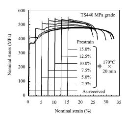
Fig.2 Stress-strain relationship of newly developed steel after strain aging
