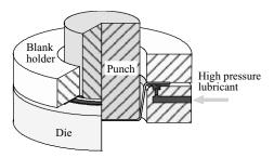
Fig. 15 High pressure liquid lubrication method
