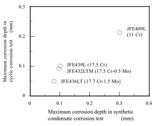
Fig.21 Comparison of corrosion resistance between steels for muffler
