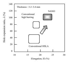
Fig.1 Comparison of El- $\lambda$  balance of 780 MPa grade hot rolled steels
