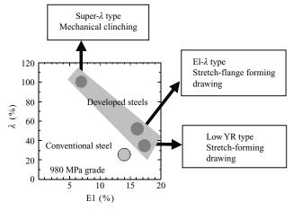
Fig.6 Typical El-*λ* balance of newly developed 980 MPa grade ultra-high strength steels
