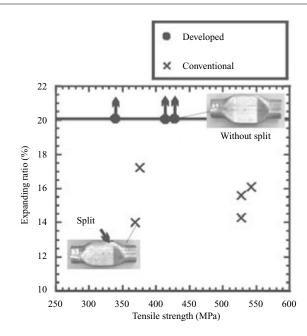
Fig.25 Relationship between tensile strength and tube hydroformability of the developed and the conventional tubes in rectangular die cavity (Maximum expanding ratio = 20%)
