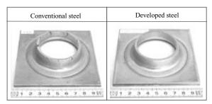
Photo 3 Hole expanded test piece (S35C)
