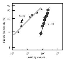
Fig.26 Rolling contact fatigue life at 180°C
