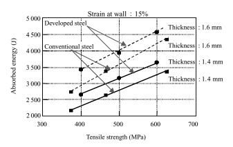
Fig.17 Improving crashworthiness of hat square column by using new developed material
