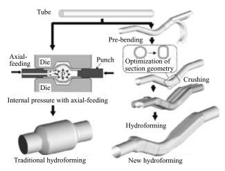
Fig.14 Manufacturing process of hydroformed tube
