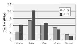
Fig.20 Core loss comparison data between JNEX and  $$\mathsf{JNHF}$$
