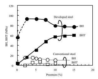
Fig.3 Effect of prestrain on BH and BHT of newly developed steel after strain aging (t = 1.4 mm)
