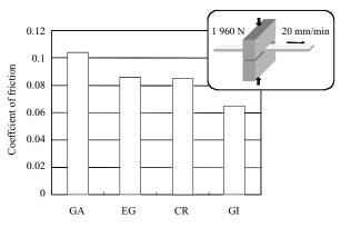
Fig.11 Influence of coating type on coefficient of friction
