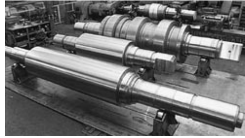
Photo 5 Rolls for hot rolling
