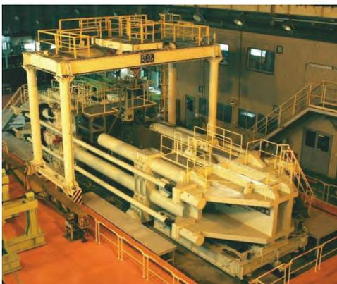
80 MN structural tensile test machine
