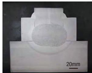
Ultra-high heat input electroslag welded joint (left) and microstructure of weld metal (right) using high-performance welding consumables
