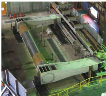
Full scale pipe bending test machine
