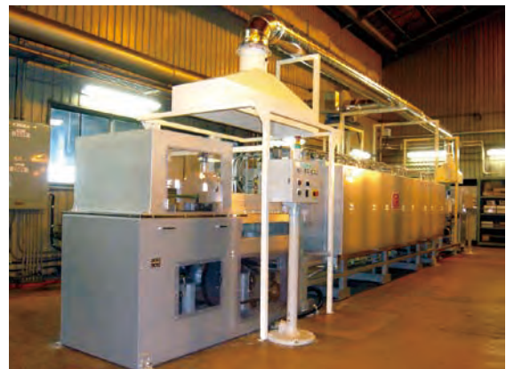
Annealing furnace for simulating final reduction process
