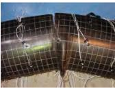
Fracture of linepipe by bending
