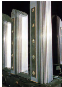
Iron core of large scale transformers of the GO electrical steel
