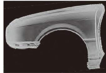
Front fender model panel ("JAZ™" JFE Zn coated steel sheet with excellent lubrication)
