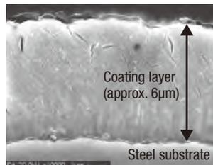
Cross sectional image of Hot-dip galvanized coating
