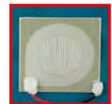
Corrosion monitoring sensor
