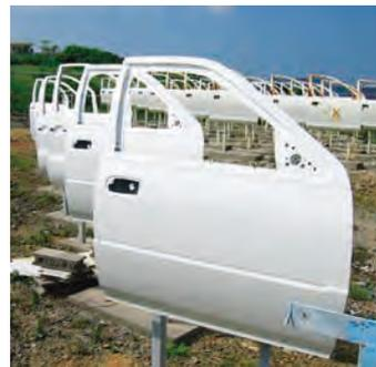
Atmospheric exposure test of actual automobile door parts (in Okinawa)
