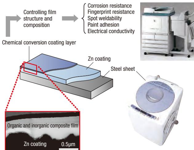
Cross section of chemical conversion on zinc coating
