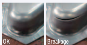
The effect of JIM-Form® on improvement of formability (590MPa HITEN)
