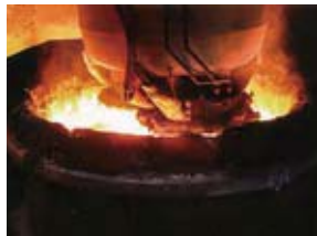
Vacuum degassing equipment
