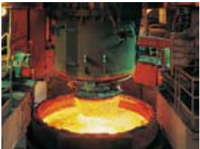
Vacuum degassing equipment
