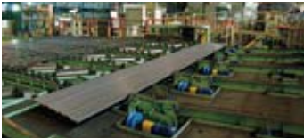
Steel bar conditioning line
