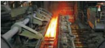
Rough rolling mill
