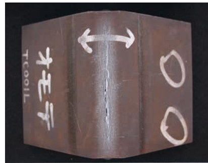
Example of crack which occurred during bending
