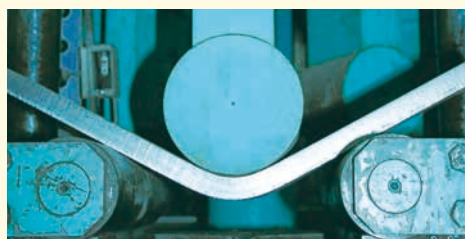
Geometry of bending test piece (JIS Z 2248)
