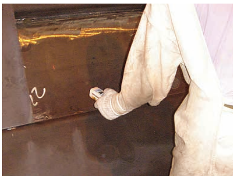
Example of temperature measurement by using a noncontact type thermometer
