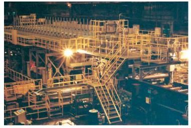
Super-OLAC<sup>™</sup> is a leading-edge TMCP technology and offers a higher cooling rate than conventiona cooling systems. Good reduction of carbon equivalent offers high weldability and improves the reliability of structures.
