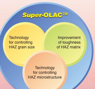
EWEL<sup>TM</sup> is composed of three independent technologies based on *Super*-OLAC<sup>TM</sup>. One of them produces finer austenite grains at the peak temperature of welding, one changes the brittle coarse bainite structure to fine ferrite and bainite structure, and the third improves the toughness of the HAZ matrix by reducing free nitrogen through chemical reaction during the welding thermal cycle.
