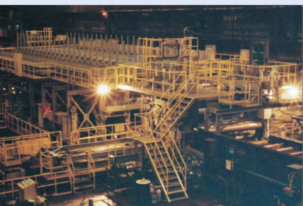
Super-OLAC™ (Online accelerated cooling equipment)
