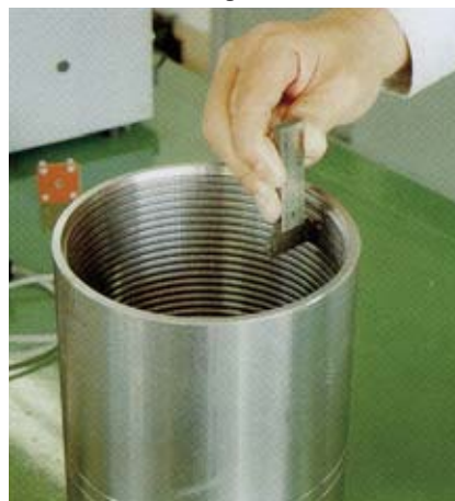
Go/No-Go Gauge to inspect thread form.
