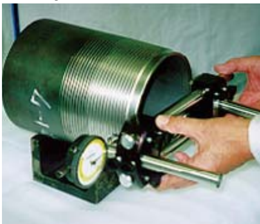
To measure thread diameter.
