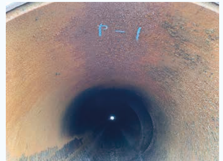
Inside surface of cargo oil pipe (17.5 years in service)
