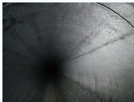
Inside surface of cargo oil pipe (15 years in service)
