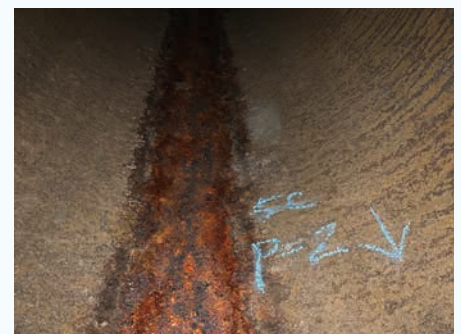
Inside surface of cargo oil pipe (17.5 years in service)
