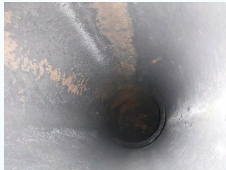
Inside surface of cargo oil pipe (15 years in service)
