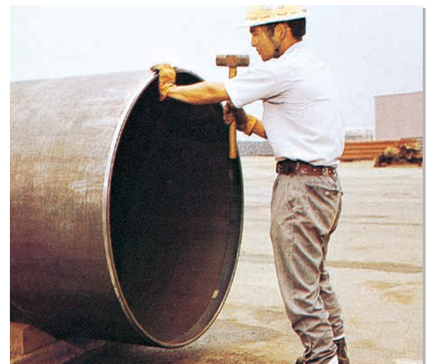
Installation of bevel protector (in sequence from top to bottom)
