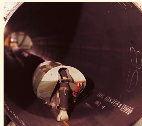
Automatic inside submerged arc welder
