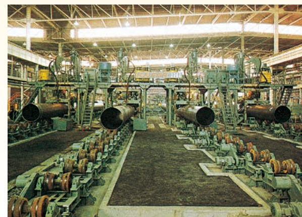
Automatic outside submerged arc welders
