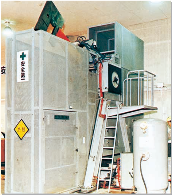
Large-scale impact tester (for DWTT and DT-test)
