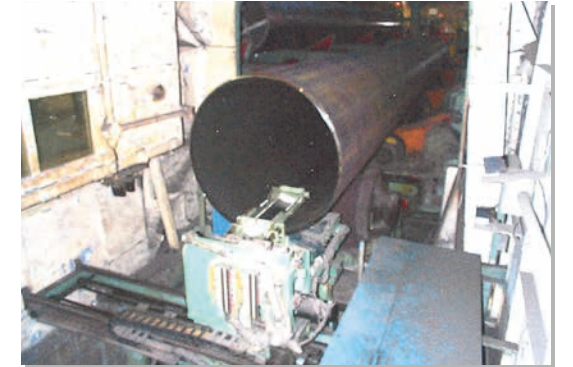
X-Ray equipment for pipe ends
