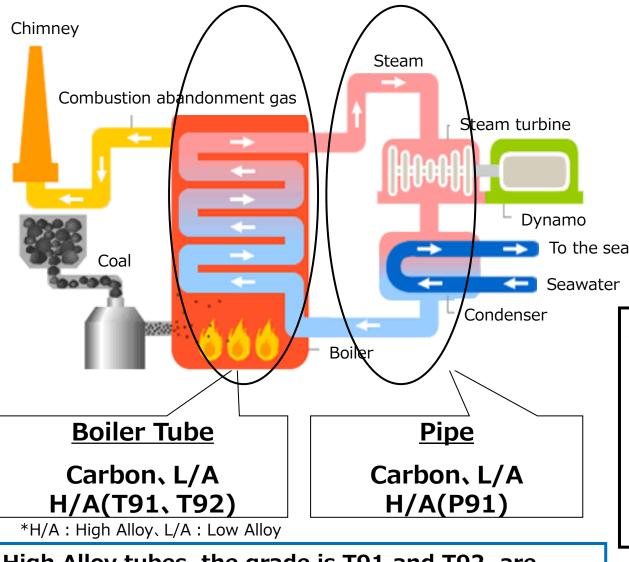
High Alloy tubes, the grade is T91 and T92, are enable to use at high temperatures and pressure for long periods of time.
