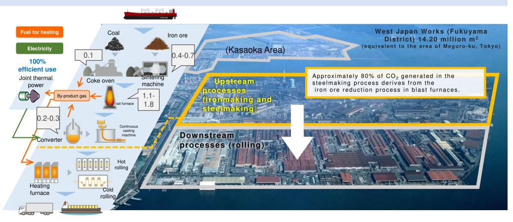
$^{\ast}$  The numbers in the diagram indicate the CO\_2 emissions intensity (t- CO\_2 /t) in each process.
