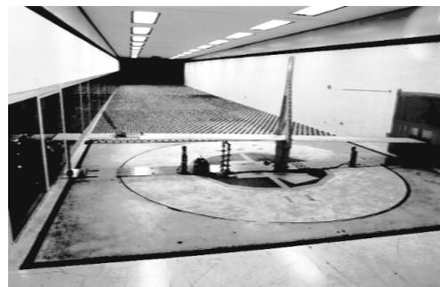
Photo 4 Wind tunnel test for the aerodynamic study on a cable-stayed bridge under construction
