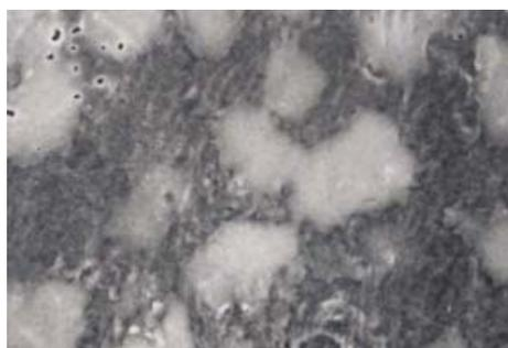
Photo 3 Scanning electron micrograph of Litewel-N
