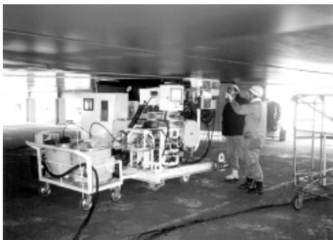
Photo 1 Automatic welding of ship's shell plates
