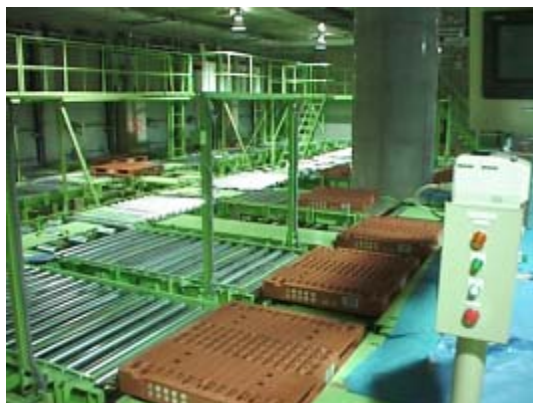
Photo 3 Pallet sorter picking system
