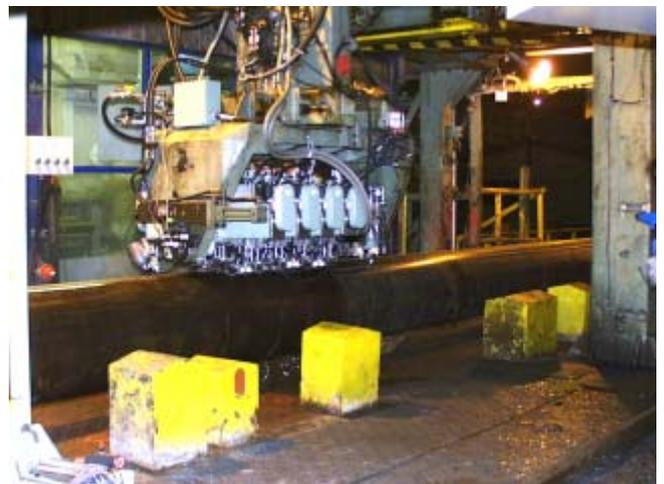
Photo 1 View of the automatic ultrasonic inspection system for weld seam of UOE pipe
