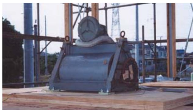
Photo 3 Vibration generator for vibration test
