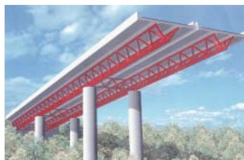
Fig.1 Image of a pipe-truss bridge
