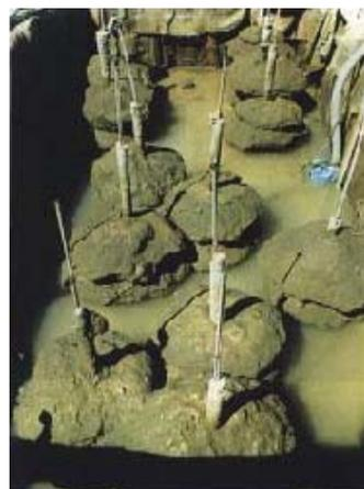
**Photo 2** Improved soil formed from grouting test using a large container
