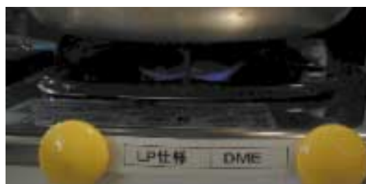
(a) LPG specification, damper opening: fixed
