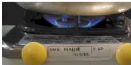
(b) 13A specification, damper opening: 8/10
