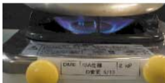
(c) 13A specification, damper opening: 5/10
