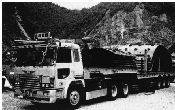
Photo 1 Transportation of inner covering plates
