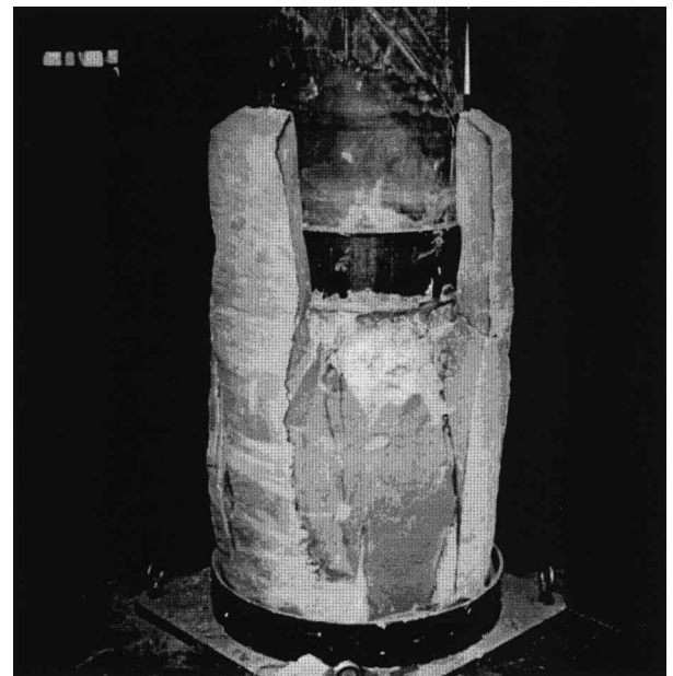
Photo 1 Failure situation of tip protection
