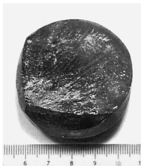
Photo 2 PZNT crystal of 100% single crystal ratio (50 mm in diameter)
