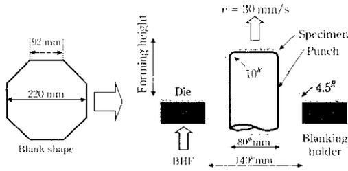
Fig. 4 Conic trapezoid shape forming test method
