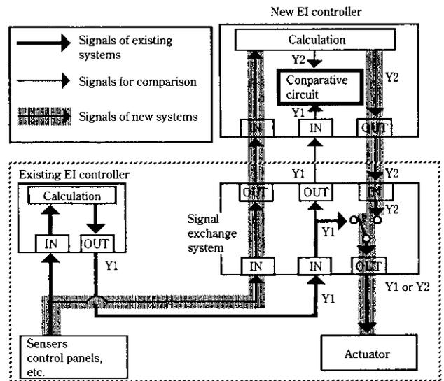
Fig. 3 Signal flow of parallel running test
