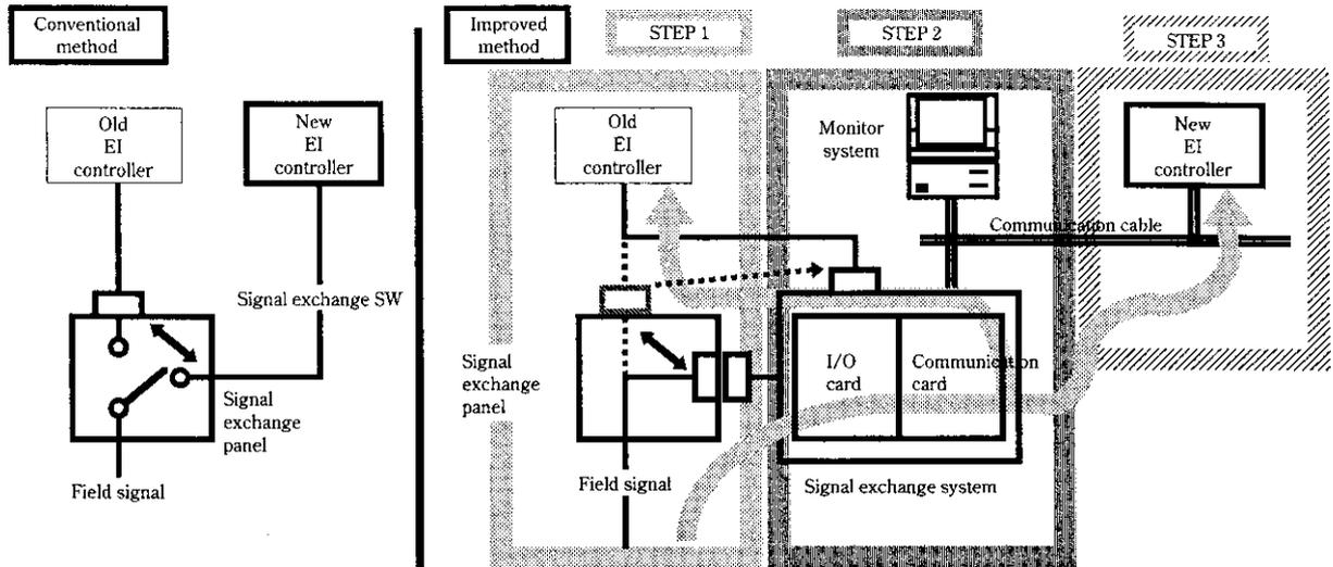
Fig. 2 Replacing technique and step of replacement
