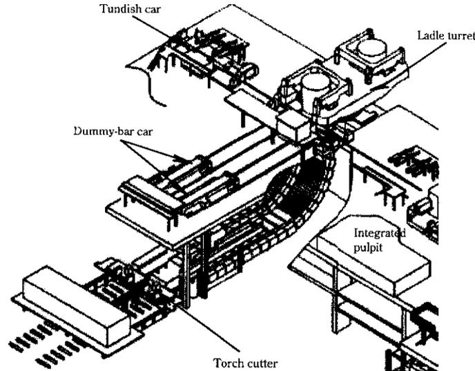
Fig. 1 Schematic view of No. 3 continuous casting machine
