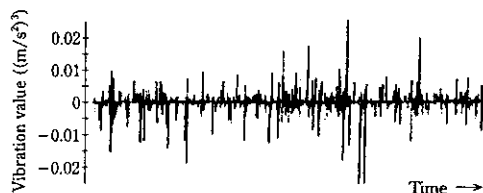
Fig. 4 Treatment wave form of the abnormal bearing
