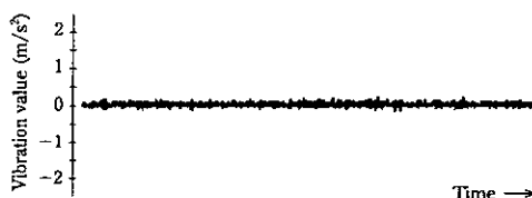
Fig. 2 Original wave form of the abnormal bearing
