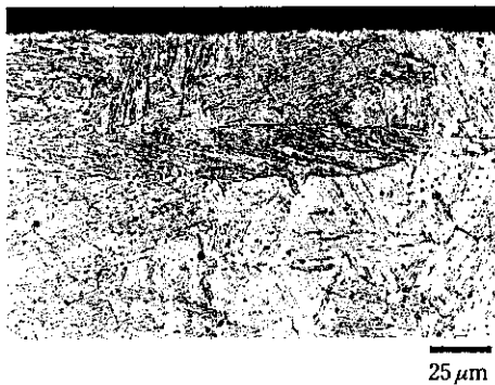
Photo 4 Microstructure of test piece of material C at the outer layer after exposed steam test under a condition of 700°C × 96 h
