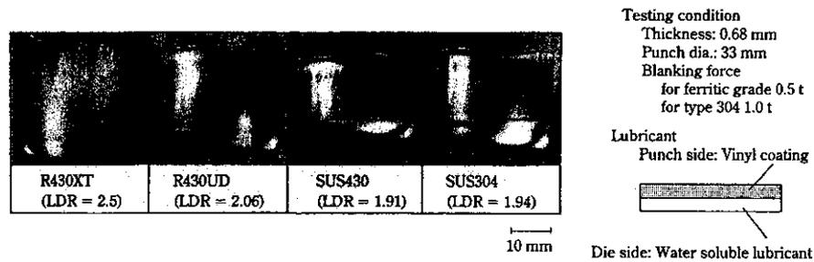
Photo 5 Appearance of ridging and drawn cup-height of R430UD and R430XT after Olsen cup test
