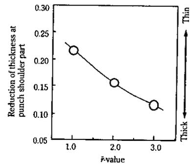
Fig. 5 Effect of r-value on the reduction of sheet thickness at punch shoulder part
