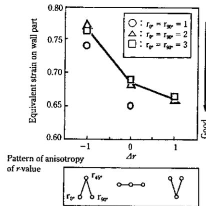
Fig. 6 Effect of Δr on equivalent strain on wall part
