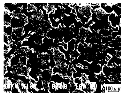
Photo 1 Surface of dull finish "Silver Soft" observed by SEM
