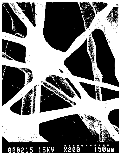
Photo 1 Structure of KP sheet (expansion molding)
