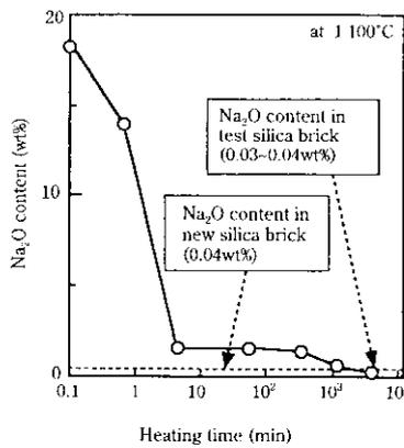
Fig. 5  $\text{Na}_2\text{O}$  content in the glass coating layer
