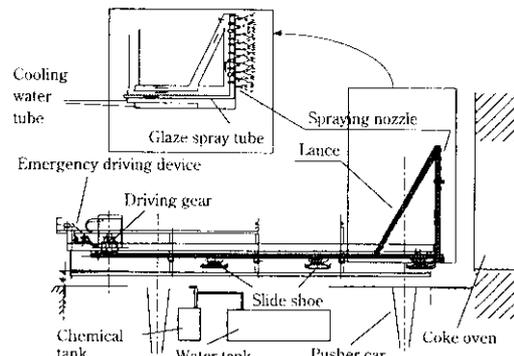
Fig. 6 Spraying equipment
