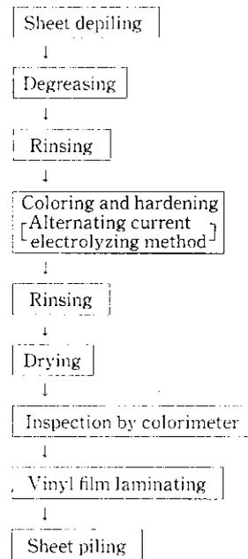
Fig. 3 Coloring process
